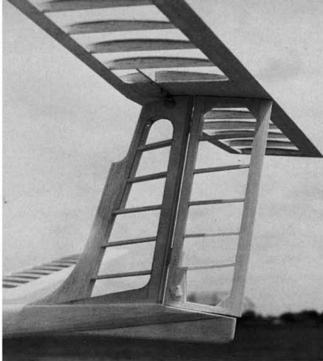
Stabilizer sits atop the fin. Note antenna hooked to hinge mount screw. Left: A flex cable fits inside fin leading edge to fly the stabilizer. Below: The structure ready for covering. Stab is sparless to keep light.
