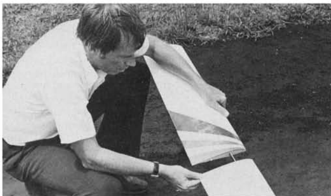
The aluminum joiner slides into spar boxes. Dowel keeps panels in line. Below: Outer wing panels plug on. Scotch tape secures them in position. A gentle, snug fit. Leading and trailing edge must line up accurately.
